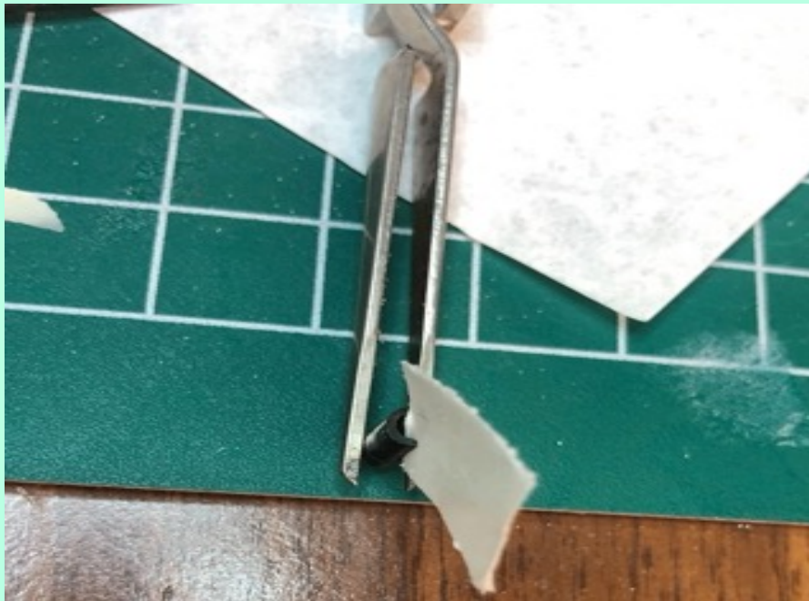
Figure 2. A thin piece of styrene has been inserted in the radial break in the Bowser #1291. Replacing the #1291 solved the problem!
